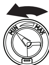
Counterclockwise to reduce foaming
