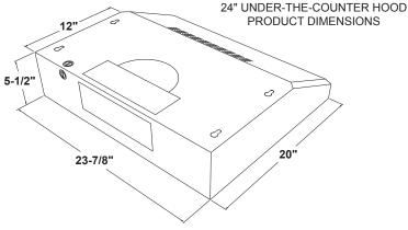
Exhaust outlet connects to  $3\text{-}1/4" \times 10"$  rectangular duct. Vent top or rear. Includes rectangular damper.
