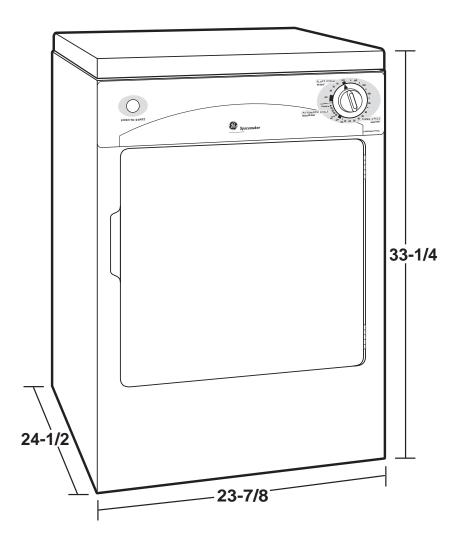
**Dryer Note:** Dryer wall outlet must be located within 36" of service cord entry and accessible when dryer is mounted in position.
